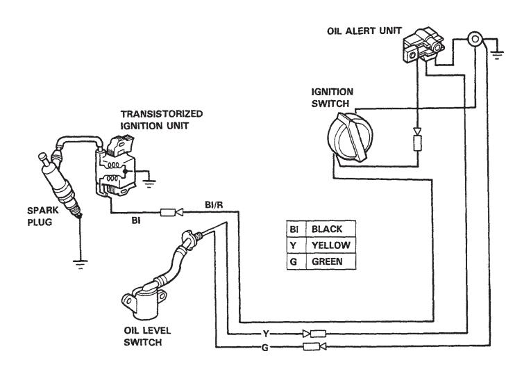
Figure 52. 13HP Honda Engine Wiring Diagram
